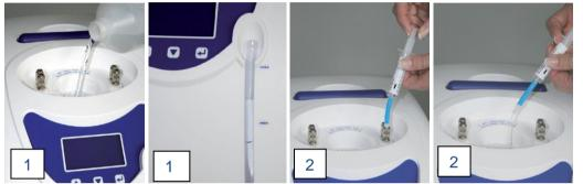
2. Remove any air from the device. Click the deairing set into the coupling on the top of the device. Pull the syringe until water is sucked into the deairing set. Remove the deairing set and empty the syringe back into the water tank. Repeat until only water (no air) is removed from all connectors.
