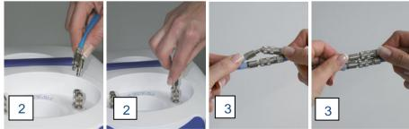
3. Connect cuff(s) to the hose(s). Insert the plug-in nipples of the cuff into the connection couplings of the hose. Make sure it is firmly connected. It doesn't matter which plug is plugged into which coupling.
